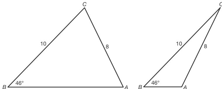
$$\frac{10}{\sin(\angle A)} = \frac{8}{\sin(46^\circ)} \text{ geeft } \sin(\angle A) = \frac{10 \cdot \sin(46^\circ)}{8} \text{ dus } \angle A = 64,0\dots^\circ.$$
