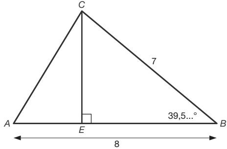
In  $\triangle BCE$  is  $\sin(39,5\dots^\circ) = \frac{CE}{7}$ , dus  $CE = 7 \sin(39,5\dots^\circ) = 4,45\dots$
